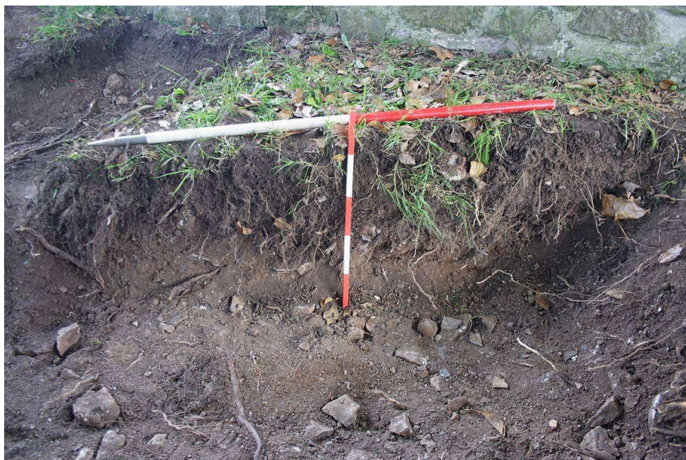
Photo 9: Typical section of investigation pits examining spread of tree roots, 1m & 0.5m scale
