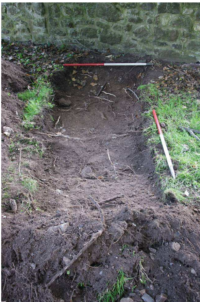
Photo 7: View looking south at one of the investigation pits examining the extent of root action around the trees
