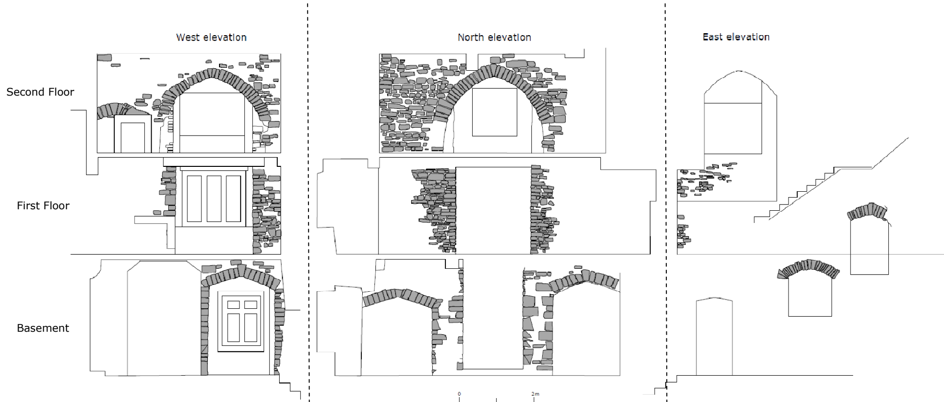
Figure 9: Elevation drawings showing west, north and east elevations of northern end of D-Shaped Tower for Basement, First and Second Floors
