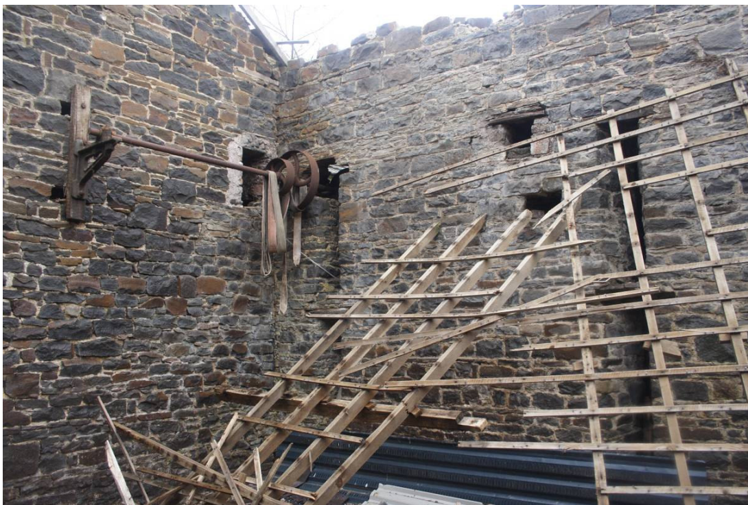
Photo 19: Remains of belt driven machinery within Building 4. Access opening connecting belts to possible wheelhouse visible behind drive wheels
